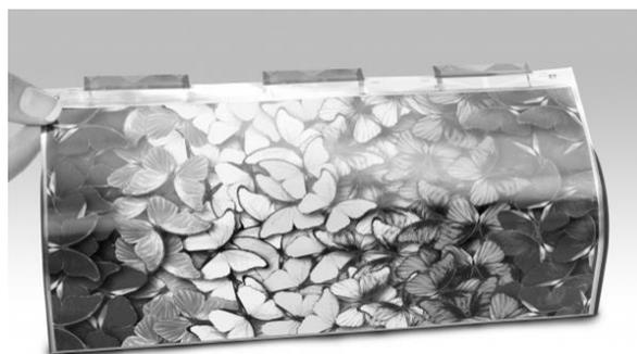
图 8. PlayNitride 与 AUO 合作, 9.4-inch, 5.5M 30um Micro-LED, 228 PPI, LTPS TFT plastic backplane
